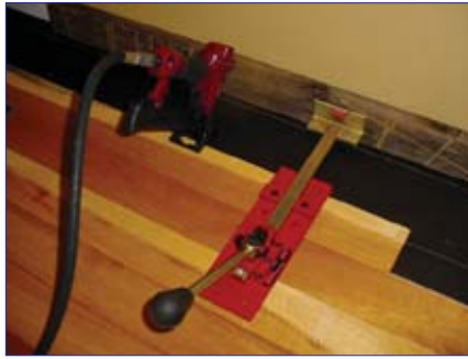
The PortaJack, locked in position, holding the board tight.
